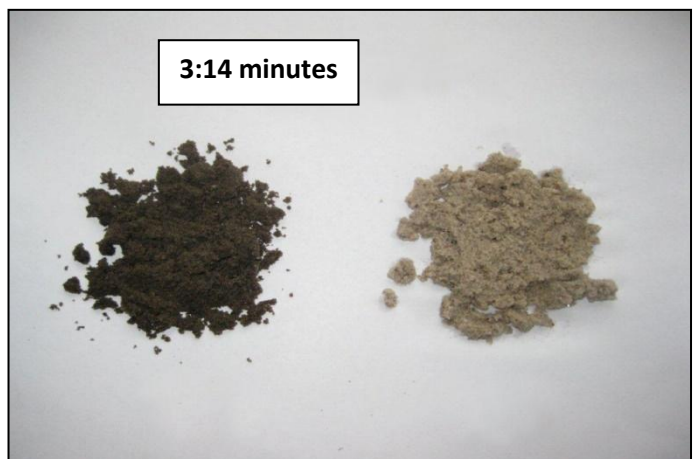
Left: Oil contaminated sand before cleaning Accell® Clean, right same sand after cleaning with Accell® Clean SWA, 3:14 min later.
